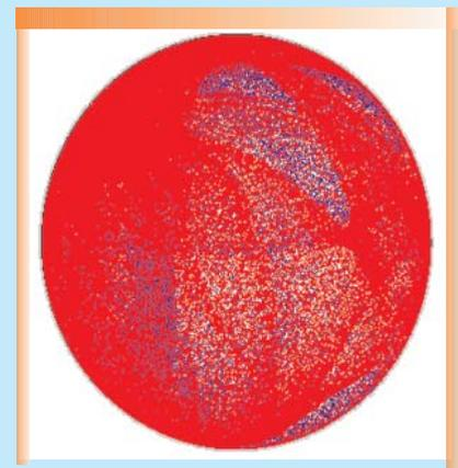
**Figure 2: 3-Cell/4-Cell Polarization Scrambler Output**
